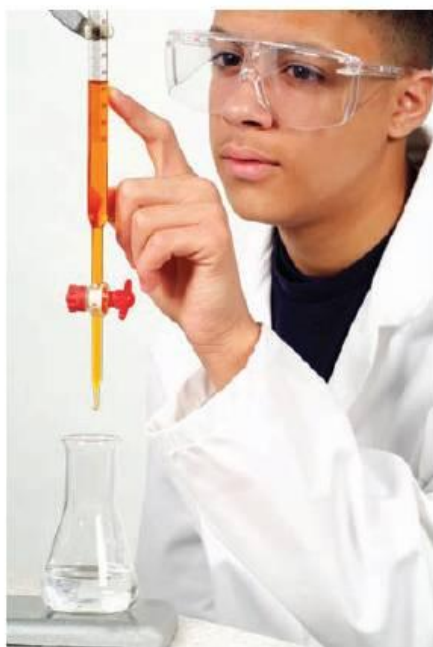
Figure 6.4 When reading a burette, the volume noted is the level of the bottom of the meniscus. What are the two burette readings, and what volume has been run out of the burette shown in the photographs?
