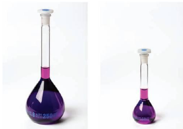
Figure 1.11 Colour is related to concentration, an intensive property that does not depend on how much solution there is.
