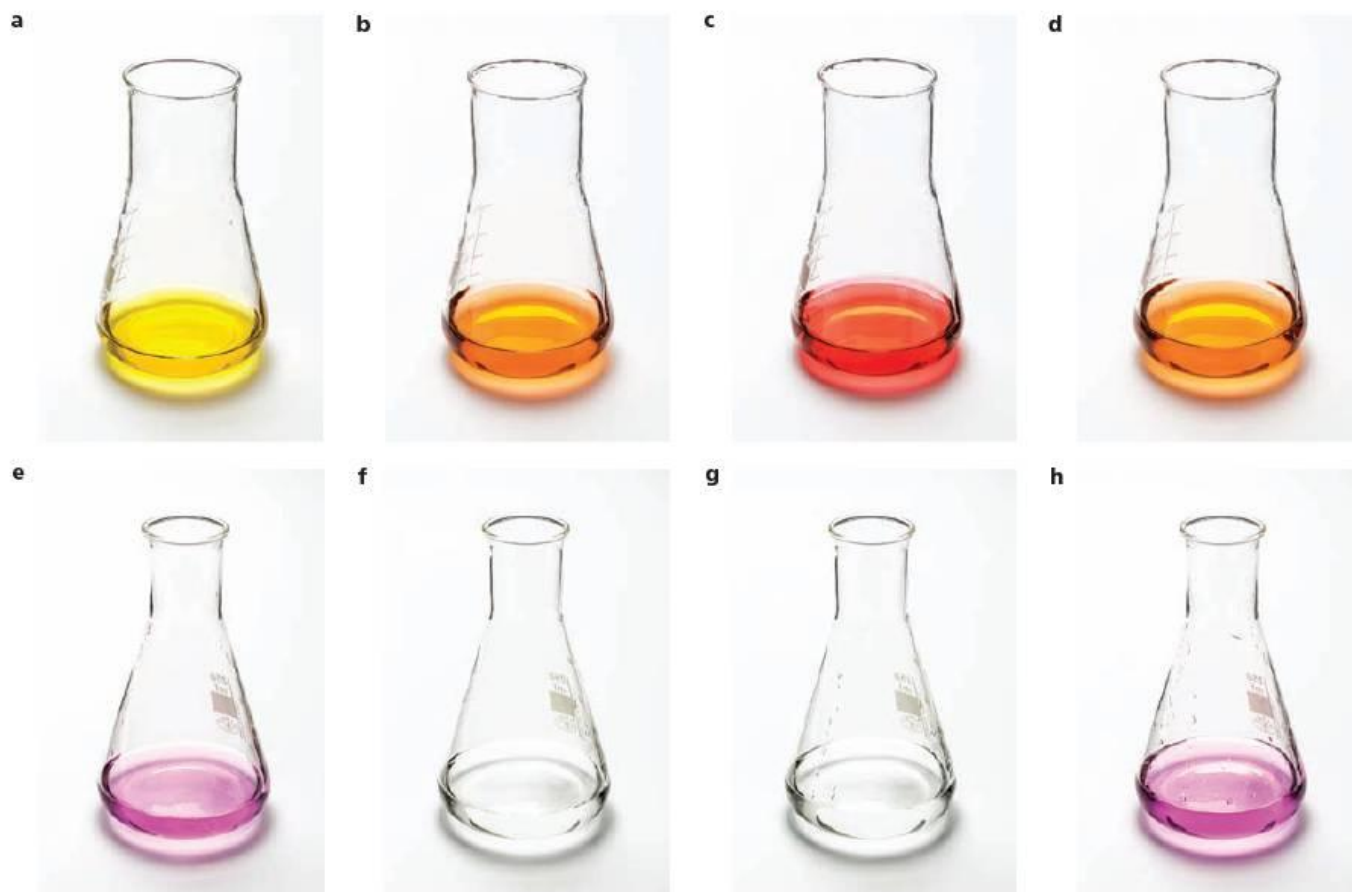
Figure 6.5 The colour changes of methyl orange (a → b and c → d) and phenolphthalein (e → f and g → h) at the end-point
