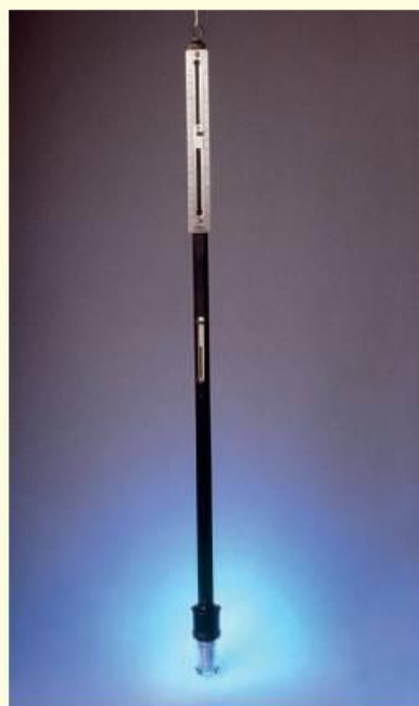
Figure 4.34 A simple barometer (left) and the vernier scale used to read the height to the nearest 0.1 mm
