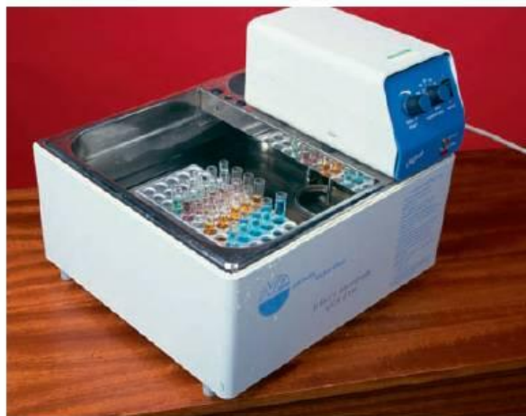
Figure 21.2 A thermostatic water bath keeps the temperature of the reaction constant, removing one factor that might affect the rate.
