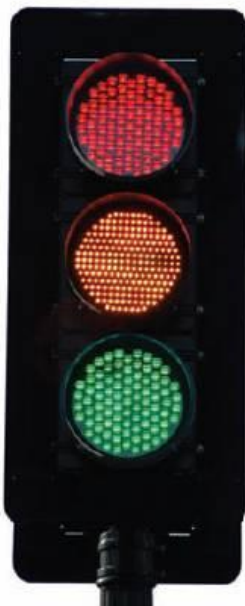
Figure 28.20 Red, yellow and green OP-LED used in traffic lights
