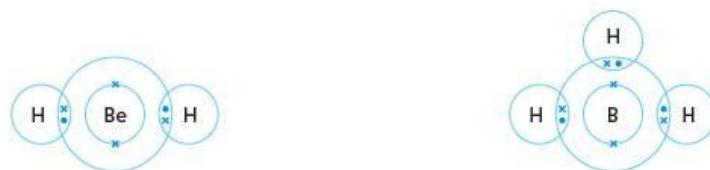
Figure 3.4 Dot-and-cross diagrams showing beryllium hydride, \text{BeH}_2 , and boron hydride, \text{BH}_3 . (It is worth remembering that all electrons are identical, no matter which atom they came from. Our representing them as dots and crosses is merely for our own benefit, to make it clear to us which atom they were originally associated with.)
