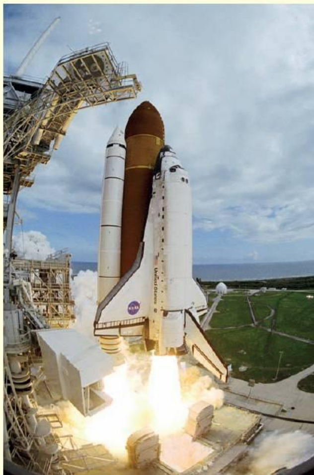
Figure 5.10 The solid fuel boosters of this spacecraft burn ammonium chlorate(VII) and aluminium. Clouds of aluminium oxide are produced as well as the gases that propel the craft into space.
