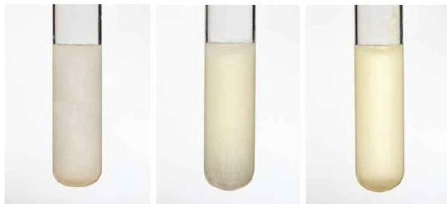
Figure 11.1 The colours of the silver halides are used in tests for the halide ions.
