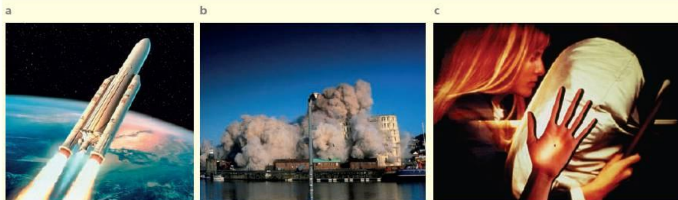
Figure 20.14 a Ariane rocket. Liquid hydrogen is used as fuel in the rocket engine. The two rocket boosters either side of the main body add to the thrust of the engine. b High explosive is used to demolish this warehouse. c Airbags in cars require rapid release of nitrogen to inflate.
