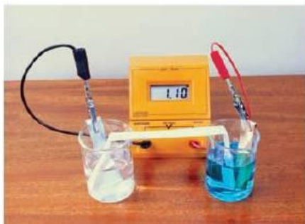
Figure 23.3 Copper and zinc half-cells connected together
