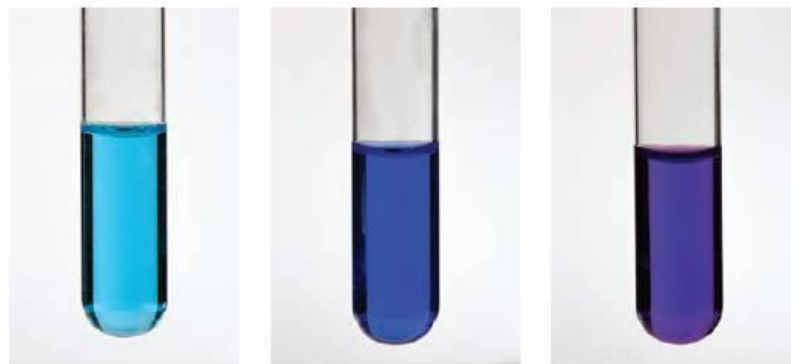
Figure 24.16 Colours of some \text{Cu}^{2+} compounds. As the ligand field becomes stronger, the splitting between the d orbitals increases and the absorption moves from the infrared into the visible region of the spectrum.
