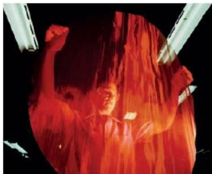
Figure 8.15 A catalyst in the form of a gauze. This provides a large surface area, but prevents the catalyst being swept away in the stream of gases.
