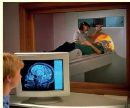
Figure 29.20 A magnetic resonance imaging (MRI) scanner gives a three-dimensional picture of the inside of the body, allowing non-invasive diagnosis of many diseases.
