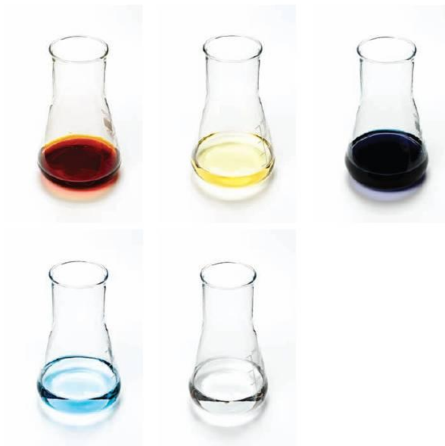
Figure 7.5 The end-point of an iodine titration is made much sharper using starch. A few drops of starch solution are added when the solution is pale yellow; the end-point occurs when the intense blue colour just disappears.
