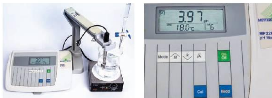
Figure 22.1 In this experimental set-up to record titration curves, the reaction mixture is stirred magnetically and the change in pH is recorded on the meter.
