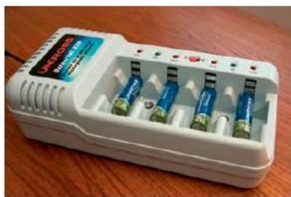
Figure 23.10 Rechargeable batteries. The chemical reactions that take place at each electrode must be reversible. Side reactions limit the number of recharging cycles that can be achieved – for most cells this is about 1000.
